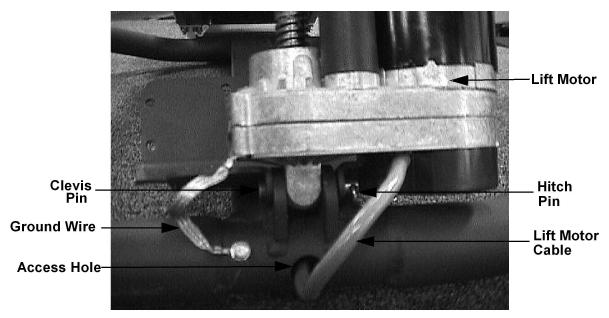
6. Remove the lift motor from the EFX.
